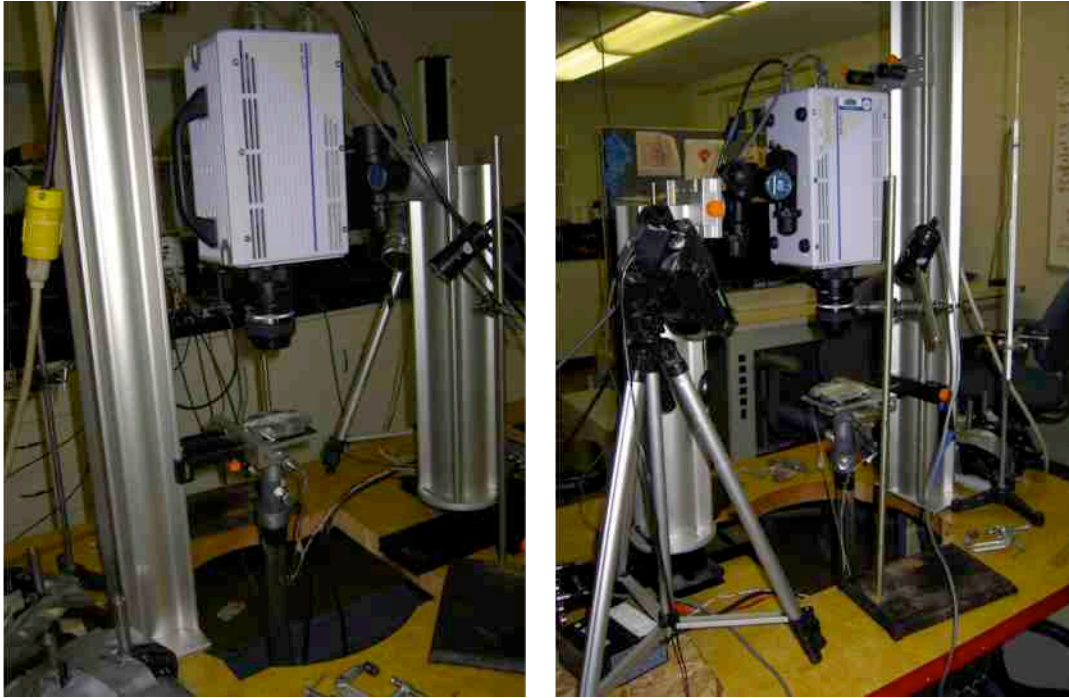
Figure 25. Photos showing the set-up and positioning for the high speed and digital video cameras used to record testing.
