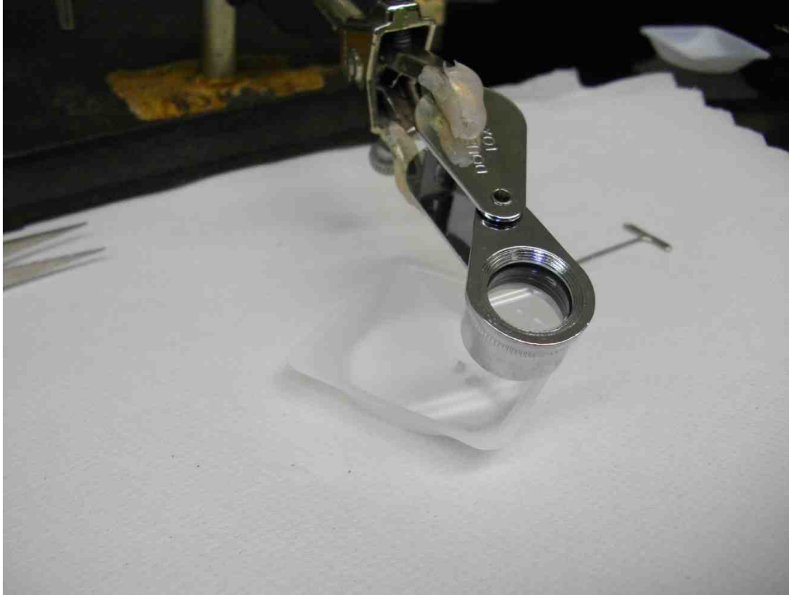
Figure 30. Set-up used to count acrylic fibers in each nonlinear fiber model. 10x magnification Selsi Loope (model No. 415) was used, as shown in this photo.
